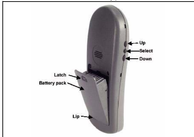
Figure 5 WLAN Handset 2210 and 2212 battery pack location
